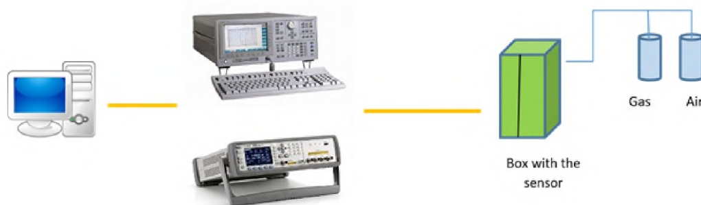
Figure 2. Installation for measurement of gas-sensitive properties of a sensor
