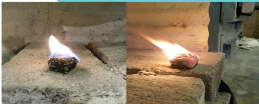
Burning of briquettes from Oi-Karagai coals with binding polyethylene terephthalate
