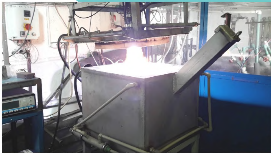
Plasma-chemical reactor with an operating electric arc plasmatron
