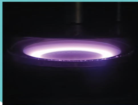
Figure 2. Argon ion discharge plasma in a magnetron used for the synthesis of diamond-like films modified with nanoparticles of different metals
